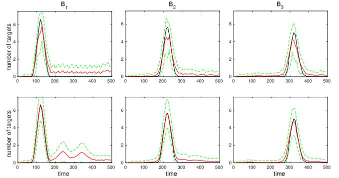
Fig. 2: Estimated target activity for naive (top) and variance-based (bottom) controllers ( $p_d = 0.6$ ,  $\lambda_{fa} = 1$ ). True target number is in black, mean target number is in red, +/- standard deviation is in green.
