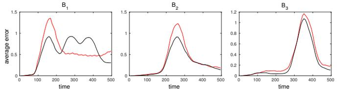
Fig. 3: Absolute error in target number ( $p_d = 0.6$ ,  $\lambda_{fa} = 1$ ). Naive controller is in red, variance-based controller is in black.
