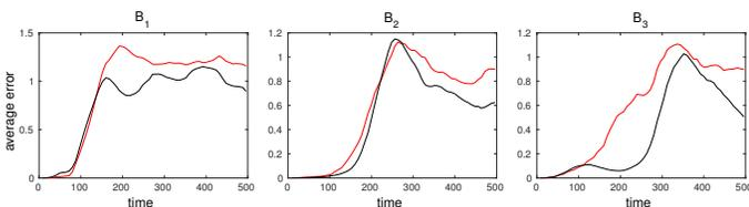
Fig. 5: Absolute error in target number ( $p_d = 0.8$ ,  $\lambda_{fa} = 10$ ). Naive controller is in red, variance-based controller is in black.
