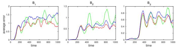
Fig. 6: Absolute error in target number ( $p_d = 0.8$ ,  $\lambda_{fa} = 1$ ).  $\lambda_b = 0.05$  is in green,  $\lambda_b = 1$  is in red,  $\lambda_b = 20$  is in blue.
